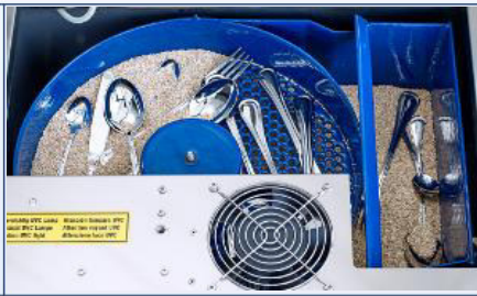
The cutlery is spirally transported upwards through a high-grade sterile granulate and is dried and polished. The installed ventilator prevents that granulate comes out of the machine.
